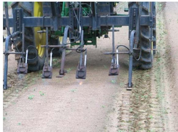
**Figure 6. Broadcast flame weeder**
