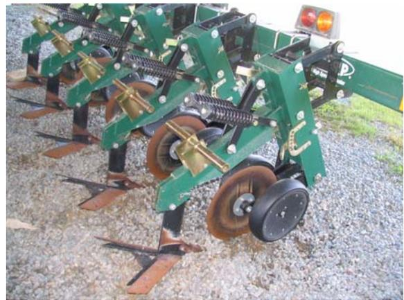
Figure 3. High residue cultivator
