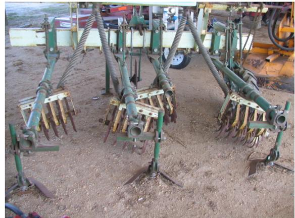
Figure 10. Rolling unit—two-row unit
